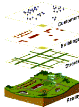
Figure 6. How does GIS work: GIS stores information about the world as a collection of thematic layers that can be linked together by geography
